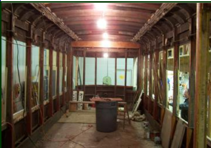
Winona No. 10 Update. The car is a shell right now except for the floor boards. A lot of the wood is already finished and in storage. Are you interested in helping put the car back together? (Jim Vaitkunas photo)
