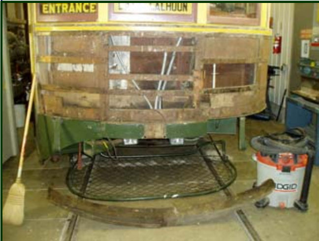
Front end exposed! Last fall here's how No. 1300's front end looked after the wood siding came off. We found a lot of wood rot and rusty steel that our shop forces treated and replaced. (John Prestholdt photo)
