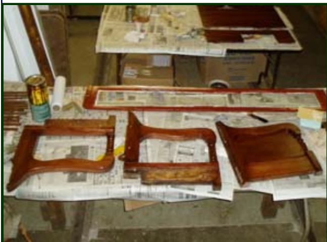
Shop Work never ends! Or—if it's not one thing, it's another department. No sooner did the major work get done on No. 1300 than our shop forces started work on refinishing pieces of Duluth No. 265 that were showing signs of wear and tear. Here we see some of the wood ends of No. 265's "peanut seats" being refinished. (John Prestholdt photo)
