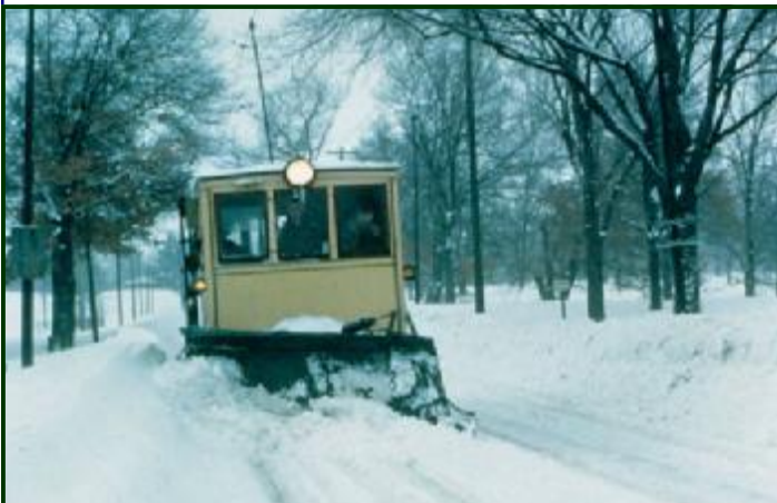
(Upper Left) A rare color photo of a TCRT plow earning its keep on the private right-of-way in Phelan Park, St. Paul.
