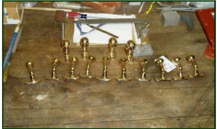
Winona No. 10 work. Our shop guys are making steady progress on Winona No. 10. Here you see brass grab handle brackets that have been machined and polished. These will look super on No. 10 when it's in service. (John Prestholdt photo)
