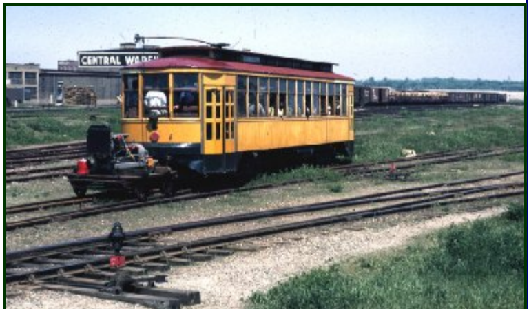
Below. Here's No. 1300 in July 1963 on a side track of the Minnesota Transfer Railway in St. Paul. No. 1300 received its electricity from the contraption shown at the rear affectionately called "the goat" which was a gasoline engine connected to a 300-volt trolley bus motor that acted as a generator. (All photos from MSM's photo archives)
