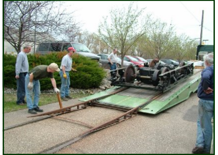
Left. The Dupont truck is unwrapped. Right. The truck is then winched down the tilt-bed trailer's ramp (Jan Albrecht photo)
