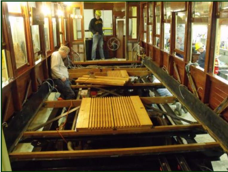
**Dick Zawacki** is shown here working on fitting the floor traps. The floor traps are removable to allow access to the motors for servicing.
