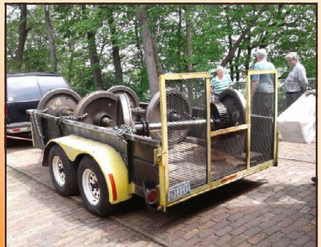
Here are three of the four axle-wheel sets ready for transport to L&S Electric in Coon Rapids, Minnesota. The other axle and wheel set was shipped to L&S previously to see if they can re-profile the wheels. The answer to that question was yes. *(Jack Bacon photo)*
