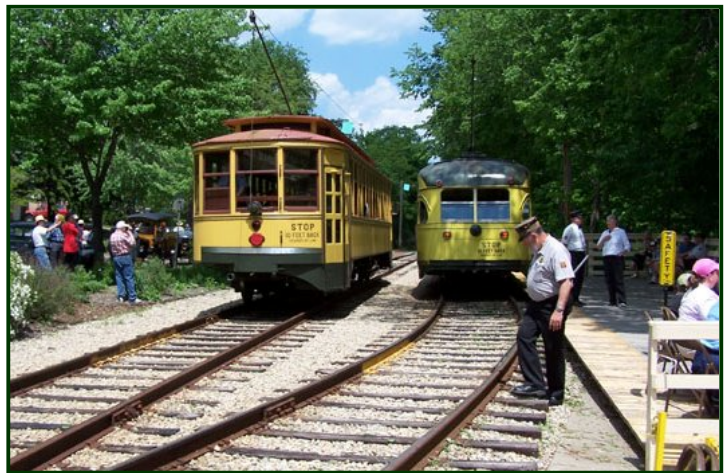
Both streetcars were busy the entire afternoon. On the right is Scott Heiderich reducing the curve noise thru grease application.
