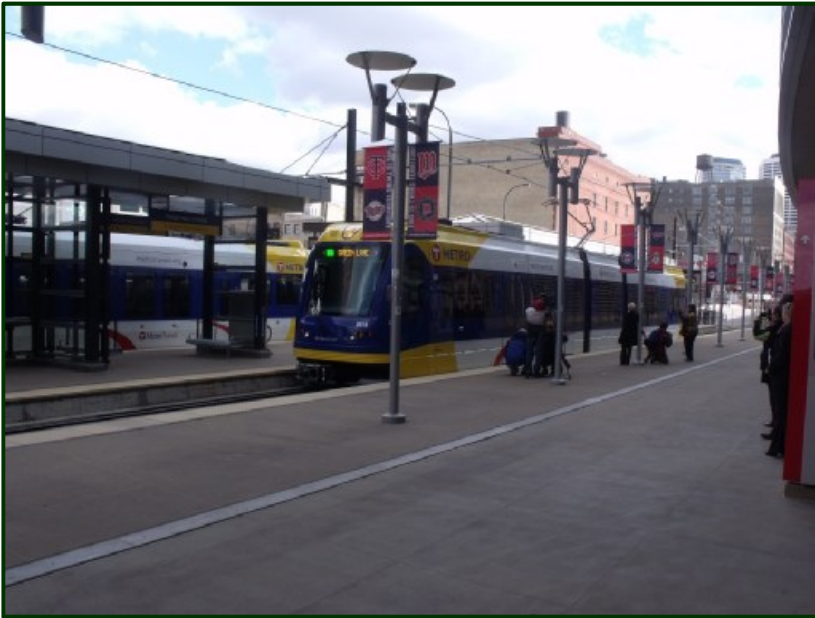
(Above) New Siemens LRV No. 201 is seen here approaching the Target Field station. Note the size of the center section which is larger than on the Bombardier-built cars currently running on the Blue Line. Reportedly the car rides much better than the Bombardier cars. (Photo by Steve Glischinski)
