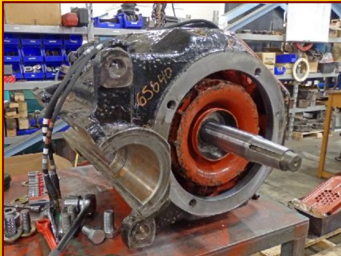
This the end of the motor armature shaft where the pinion goes.
