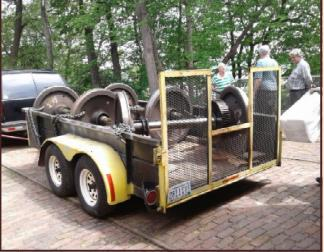
Here are three of the four axle-wheel sets ready for transport to L&S Electric in Coon Rapids, Minnesota. The other axle and wheel set was shipped to L&S previously to see if they can reprofile the wheels. The answer to that question was yes.
