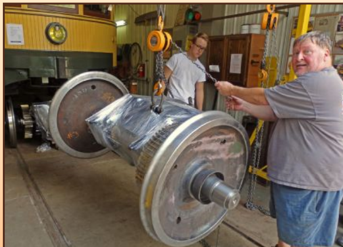
Rob Mangels, Jr. (left) and Tom Schramm position one of the axle-motor sets delivered earlier.
