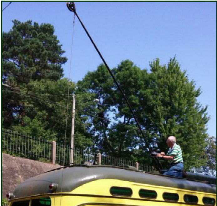
Trolley Pole Problems! Russ Isbrandt (on No. 322's roof) and Mark Digre are adjusting the spring tension on No. 322's trolley pole that just didn't want to stay on the wire. (Jim Vaitkunas photo)
