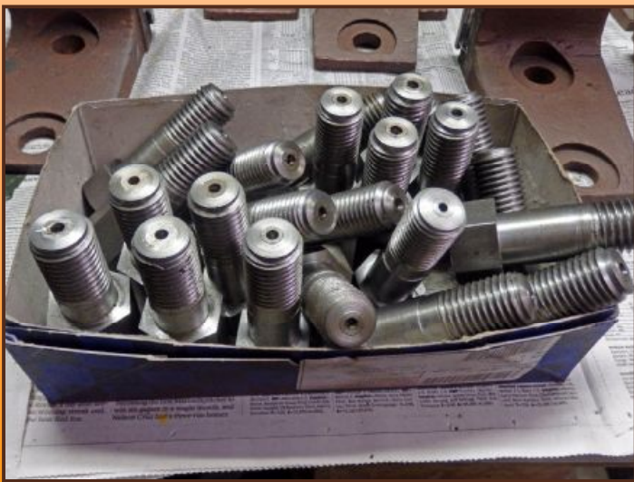
New pedestal bolts manufactured by Rob Mangels, Sr. in his shop.
