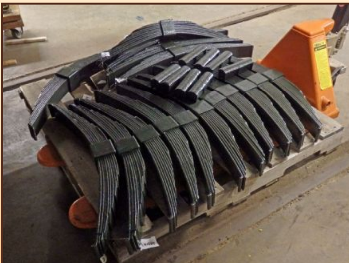
Elliptical springs ready to be re-installed
