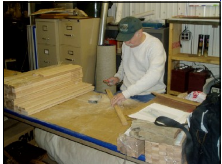
Above. Bill Arends is seen here working on some of the wooden slats that make up one of Winona 10's walk-over (flip-over) seats. Winona No. 10 is a true double-end car with duplicate controls at each end. At the end of the line, to prepare for the return trip, the Motorman swung the trolley pole around, took his control handles to the other end and flipped the seat backs over so the passengers could sit facing the front. (John Prestholdt photo)
