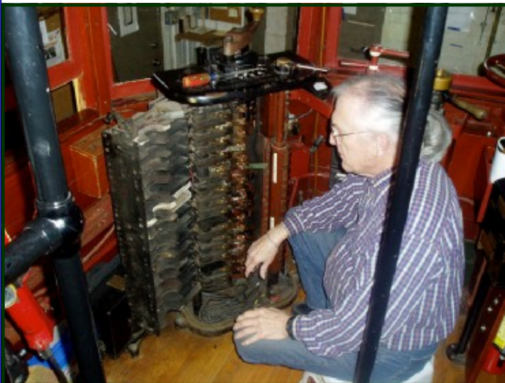
Above. Tom Fairbairn takes a quick break so the photographer can snap a picture. Here you see Duluth Street Railway No. 265's controller cover removed and the arc chutes swung aside to reveal the interior. While a streetcar controller is a relatively simple device, it still requires constant inspection and maintenance to make sure it operates properly. Our shop workers do an excellent job in taking care of our historic streetcars. (John Prestholdt photo)
