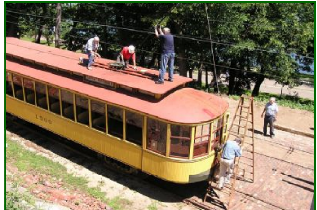
Trolley Pole Troubles. Here's most of the Tuesday crew working to replace the trolley pole on No. 1300—again. The pole broke twice in six weeks, an unusual occurrence to say the least. (Dennis Stephens photo)
