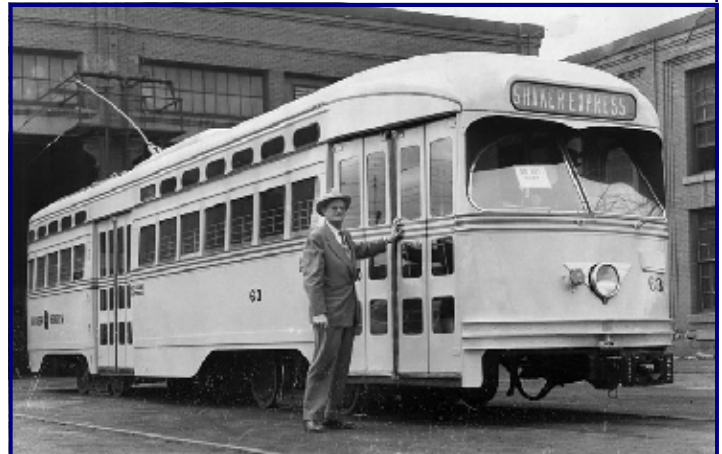
Ready for Shipping. Here's SHRT No. 63 (ex-TCRT No. 352) in SHRT colors (note SHRT's logo at the rear). Frank S. Morgan , TCRT's Superintendent of Power and Equipment, stands next to No. 63. Note the multiple unit coupler underneath the front. The sign in the window says "DO NOT HUMP" which means that the car is ready for loading onto a railroad flatcar, destination Cleveland, Ohio. (MSM Photo Archive)
