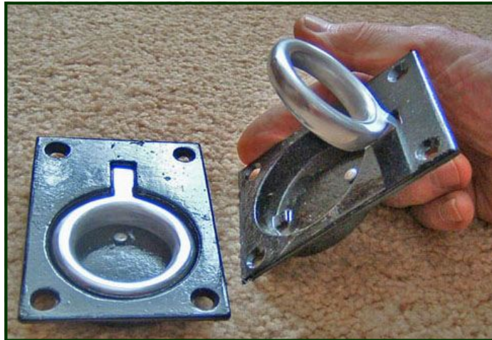
Above. These two pull rings were made by Scott Ingram . These go on the single folding leaf door located to the left of the Motorman at each end of the car. The doors were not controlled from inside the car by any kind of lever or linkage, so these pull rings were the only way to close the doors. While the doors were functional when the cars were delivered, the cars were always one-man operated. The odd doors were permanently closed and sealed only a couple of years after delivery of the four cars to the Winona system. (Photo by Ken Albrecht)
