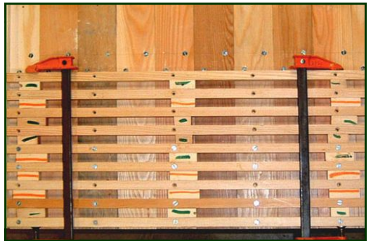
Above. This photo shows the initial work by Ken Albrecht to fabricate the grooved floor running down the middle of the aisle of Winona No. 10. This happens to be a part of a trap door to allow shop forces to do maintenance on the motors. The purpose of the grooved aisle was to allow dirt to fall between the wood runners. Women wearing shoes with any kind of heels hated this type of floor. (Ken Albrecht Photo)
