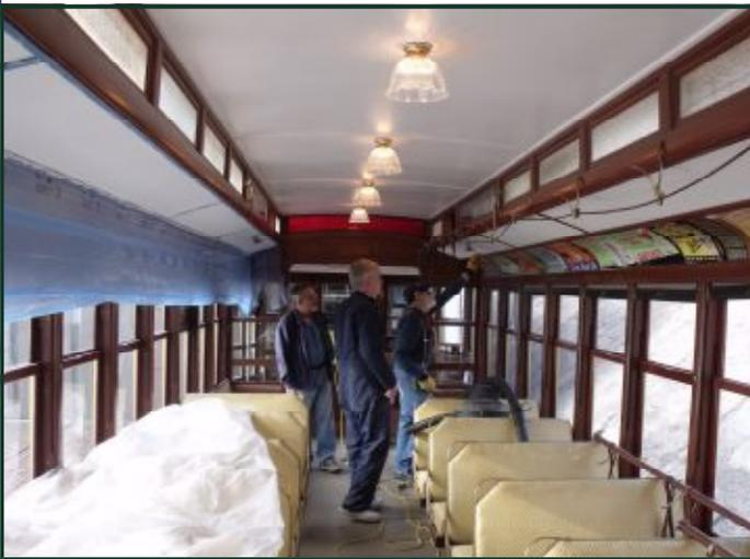
The ceiling lights are back in service in No. 1300. The top ceiling panels have been repainted and now the crew is starting to paint the side ceiling panels. Shown in the photo are (left to right) **Bob Smith, Karl Jones** and **Walt Strobel**.
