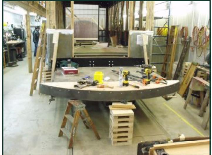
Here's a shot of one of the ends of Winona No. 10. The front part of the platform is bolted to the platform supports and the metal front bumper is screwed into that piece. You can't see them but the mortise holes are in for the platform's corner and window posts. (Photos by Jim Vaitkunas)
