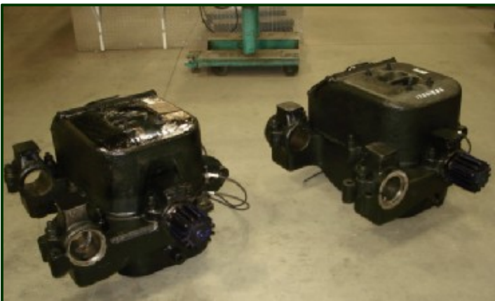
Since we rarely can see the motors that power our streetcars because they're mounted on the power truck and well hidden under the car, I thought you'd be interested in these photos of the GE-800 motors that will eventually power Winona No. 10. The photo on the left shows the motors complete with the electrical leads. The GE-800 motor is a "split-frame" type motor, and as you can see in the photo on the right, the top half of the motor case has been removed to show the refurbished armature. On the armature shaft the small pinion (gear) will mesh with a larger "bull" gear fixed to the axle. The round openings shown in the photo on the left fit around the axle so that the pinion and bull gear can mesh properly while allowing the axle to move up and down to conform to the bumps and dips in the track. Each motor weighs 1,700 pounds. It cost $13,000 to rebuild the two motors—your generous donations made it happen. Many thanks! (Photos courtesy of A.C. Electric Company, Bangor, Maine)
