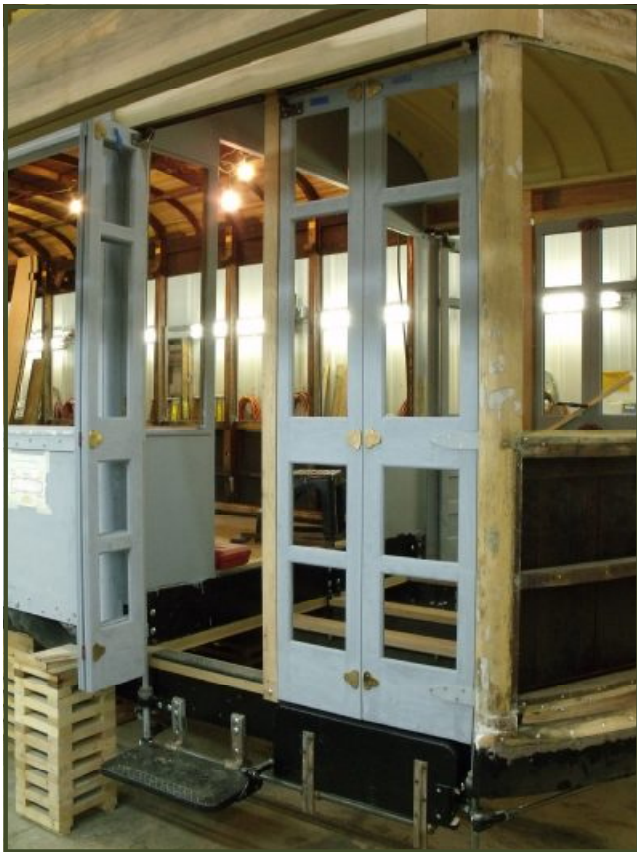
Left. Close-up of the entrance/exit doors which can be opened independent of each other. The door on the right is for boarding passengers while the door on the left is for alighting passengers. There is a single set of folding doors on the same side at the opposite end of the car that can open but do not have interior controls. These doors were permanently closed shortly after No. 10 went into service in 1914 as No. 10 never operated as a two-man streetcar.
