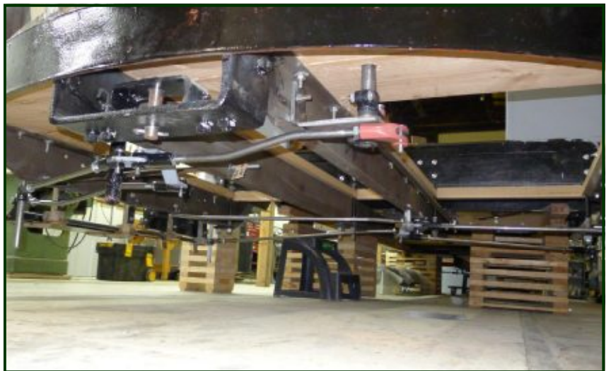
Above. Here's the underside of one of Winona No. 10's platforms. You can see (I hope) the almost dizzying array of rods, bell cranks and shafts that control the operating doors on No. 10. No. 10 was a very simple streetcar. No air-operated door engines on this car like the big TCRT "standard" cars. (Howie Melco photo)
