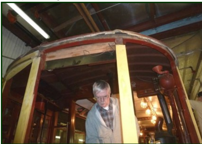
(Above left) Karl Jones works on replacing wood on the front of No. 265. (Above right) A jig was made to bend the new wood that goes around the front of No. 265. You can see where this piece will go in the left photo above the front window post (Dennis Stephens photos)
