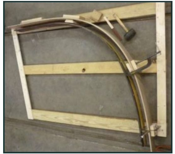
(Above left) Karl Jones works on replacing wood on the front of No. 265. (Above right) A jig was made to bend the new wood that goes around the front of No. 265. You can see where this piece will go in the left photo above the front window post (Dennis Stephens photos)
