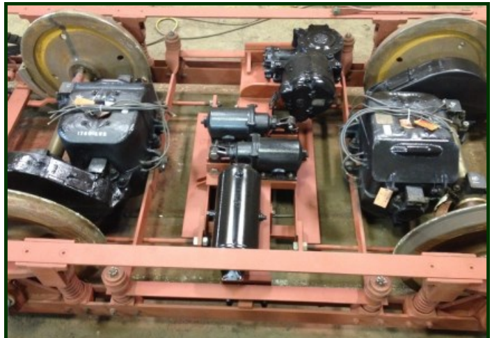
(Above left) The interior woodwork on Winona No. 10 is being put back in. (Howie Melco photo) (Above right) Lyons Industries of Ebensburg, PA has finished the truck for Winona No. 10. The black item at the top is the General Electric CP-25 air compressor. (Lyons Industries photo)
