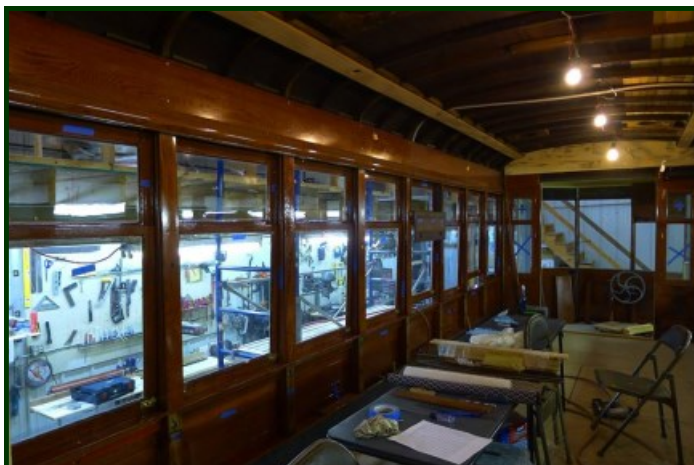
(Above left) The interior woodwork on Winona No. 10 is being put back in. (Howie Melco photo) (Above right) Lyons Industries of Ebensburg, PA has finished the truck for Winona No. 10. The black item at the top is the General Electric CP-25 air compressor. (Lyons Industries photo)
