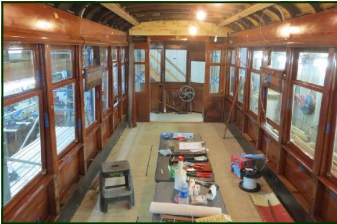
(Above left) The interior of Winona No. 10 is coming along nicely as shown in this photo. Much of the interior woodwork is finished and installed. (Above right) Scott Heiderich (left) and Mike Miller are working on the interior wiring. Here Scott is pointing to a panel above the platform entrance behind which will be mounted the fuses for the lighting and other circuits. (Bill Graham photos)
