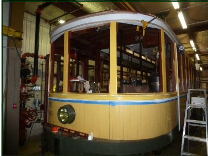
(Above left) Here's DSR No. 265's front showing good progress on the repairs. (Above right) The rear of No. 265 also required a lot of repair to rotting wood and window sash. Now we're masking off areas to be painted. (Dennis Stephens photos)
