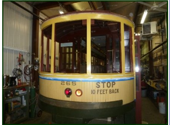
(Above left) Here's DSR No. 265's front showing good progress on the repairs. (Above right) The rear of No. 265 also required a lot of repair to rotting wood and window sash. Now we're masking off areas to be painted. (Dennis Stephens photos)
