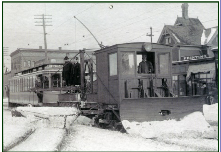
(Right) In 1905 a TCRT plow stops for a few minutes for the photographer on Nicollet Avenue just south of 31st Street in front of Nicollet Station. Everett C. Jones, a TCRT employee, is the Motorman shown in the cab. TCRT was required by its franchise to plow the streets on which it operated. A few years later the company built a fleet of more powerful and fully enclosed snow plows, capable of clearing a street in two passes. Note the open body where the wingman and Foreman must stand while operating—brrrrr. And, the front plow is made of wood slats!
