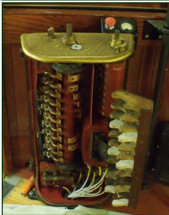
(Above) Here's a shot of the insides of a K-10 controller. The arc chute cover is moved away to show the controller's segments and fingers. Note the 600-volt wires at the bottom of the controller.
