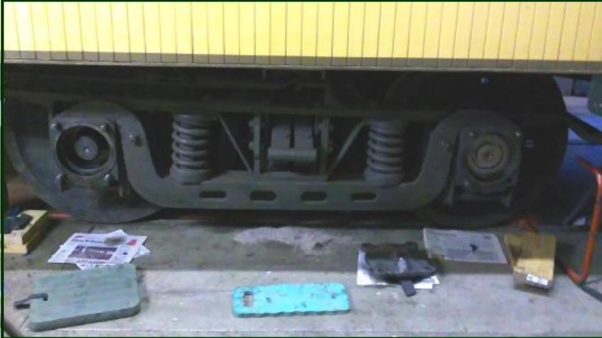
**Left.** This is a photo of the front truck under No. 1300. The culprit is the journal on the left. Near as we can tell the "race" that supports the roller bearing worked its way outward undetected over the years until it hit against the journal cover which is a steel casting. When the journal cover eventually broke we immediately took No. 1300 out of service.
