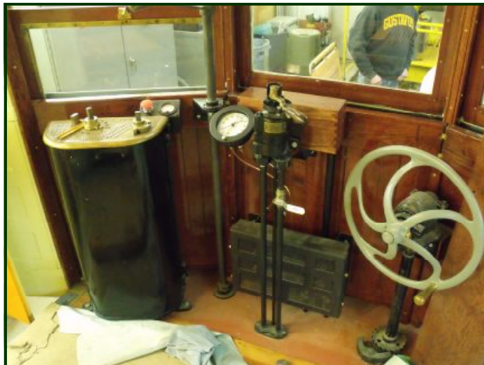
The platform controls are complete. The black thing seen on the floor to the right of the controller is a heater. No. 10 will be heated with electricity.
