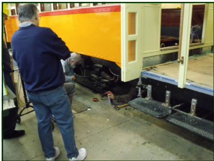
(Right) The hand reaching out from under No. 10 belongs to Howie Melco who has been working on adjusting the brake rigging. Howie is standing in the pit under the car. Art Ruder is standing in the foreground while Mark Brothen is kneeling down to hand Howie a tool.
