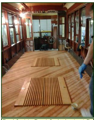
The sub floor is in. The main floor boards go in next. The main floor will continue the grooved wood shown on the floor traps. Seats will be on each side. (*Scott Heiderich photo*)
