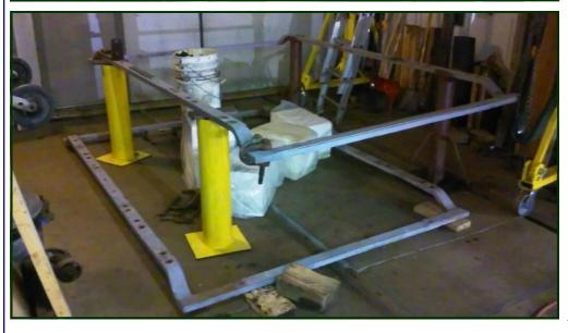
You can't dismantle a streetcar truck any more than this! These grey steel members comprise the upper frames of both trucks from No. 1300. Pedestal jaws, truck bolsters, swing links, brake rigging, etc., have been taken off for evaluation and refurbishing or replacing if they're found to be defective.
