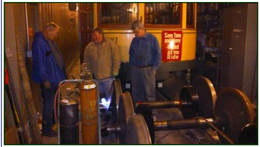
Before No. 1300's wheel sets can go to the shop so the wheels can be reprofiled, the inner roller bearing "races" needed to be taken off the axle ends. Here we see **Jim Willmore, Tom Schramm** and **Mark Digre** heating the race on one axle so it can expand and be pried-off the axle end.
