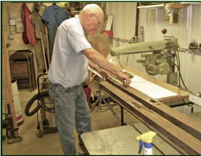
(Above) Here's Winona No. 10 Restoration Chief, Ken Albrecht working on one of the wood pieces of Winona No. 10. This was taken at the Museum's Excelsior car barn and shop and shows Ken measuring one of the replica wood pieces that was fabricated based on the original piece of wood that was damaged structurally. (Photo by Bob Johnson)
