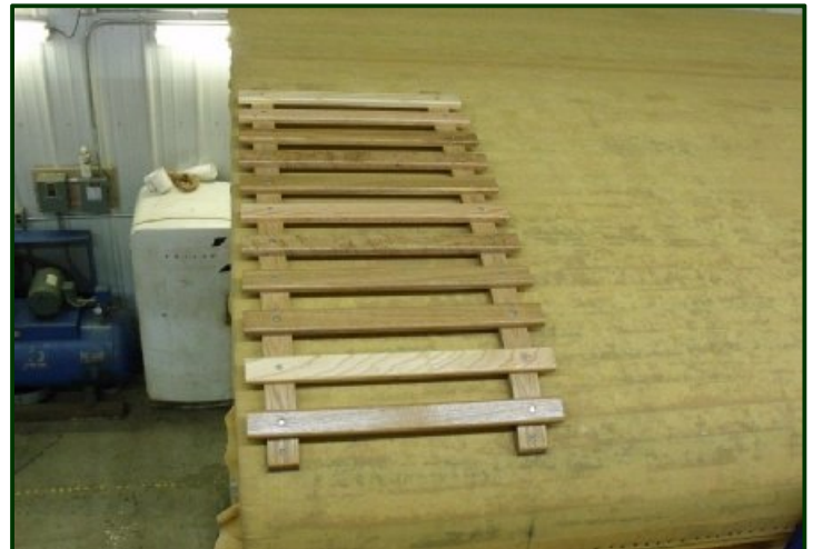
This ladder looking item is called a roof mat. A handle will go on the right side of it. This will allow someone to climb up onto the roof to make repairs to the trolley pole, for example. (Dick Zawacki photo)
