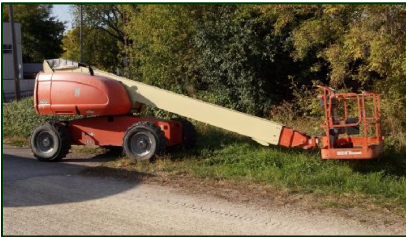
(Above) This “man-lift” machine was essential to the success of this project. As you can see from the photos in this supplement, much of the overhead work, and the tree trimming, was done away from the track in the area of the support poles. The tower wagon could not be used to work on the line poles themselves.
