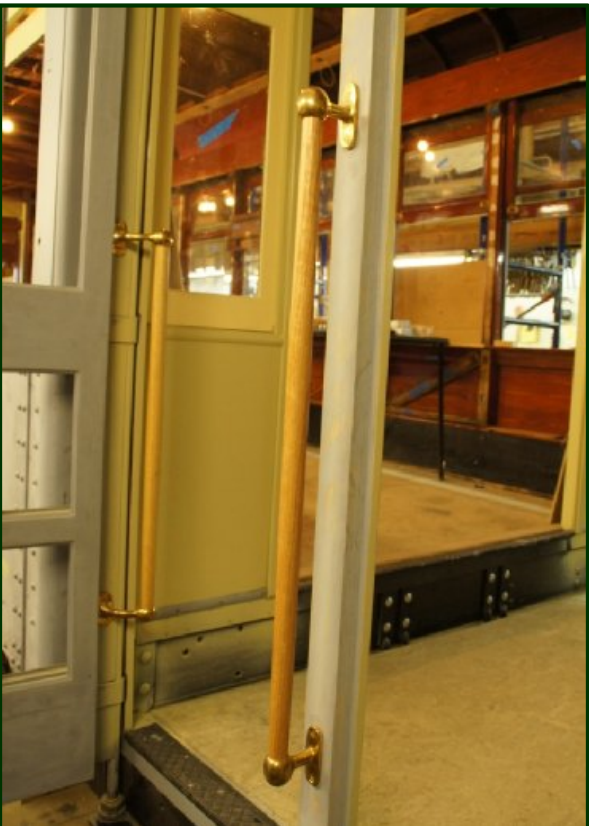
Grab bars used by passengers are shown in this photo. The interior of the platform is also primed and ready for the finish coats of paint.
