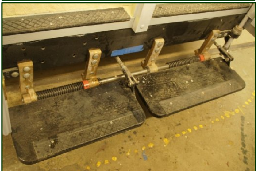
Number 10's main entrance/exit doors are to the right of the Motorman and on opposite corners of the car, as No. 10 will be a true double-ended car with duplicate controls at each end. The doors are manually operated and can be opened and closed independent of each other. The folding steps are linked to the doors so that when the doors open the steps drop down and they fold up when the doors close.
