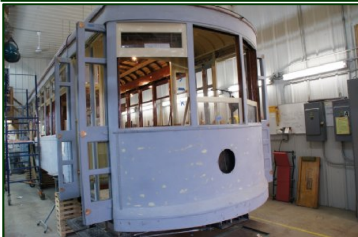
The carbody is now primed and ready for the finish coats of paint. All sash are now refurbished and ready to have the glass put in.
