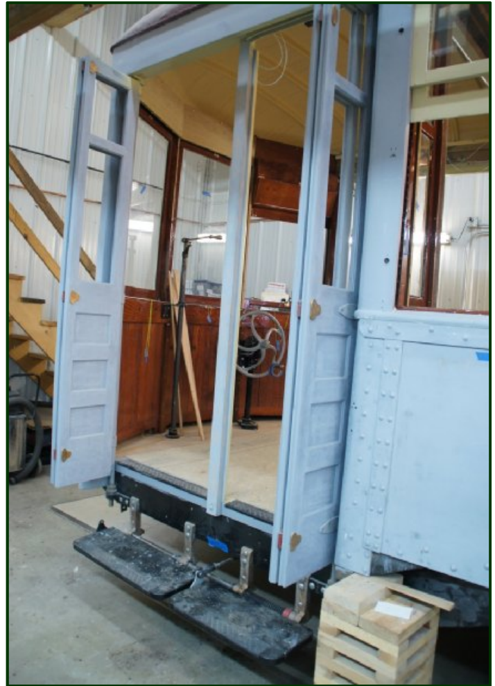
This photo shows one of the two sets of "off-side" doors and steps. One set of the doors and step to the left of the Motorman at each end of No. 10 will be permanently closed like No. 10's doors were. The doors on the right will be manually operated.
