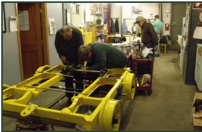
Jim Willmore & Tom Schramm working on the speeder's chain drive while John Prestholdt is working on the motor in the background. (Photo by Jim Vaitkunas)
