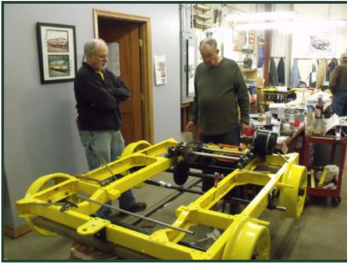
Here we see the new electric speeder's basic frame and propulsion drive. The car will be battery powered using a golf cart motor. Dennis Stephens (L) and Jim Willmore are probably discussing the triple-reduction chain drive. (Photo by Jim Vaitkunas)
