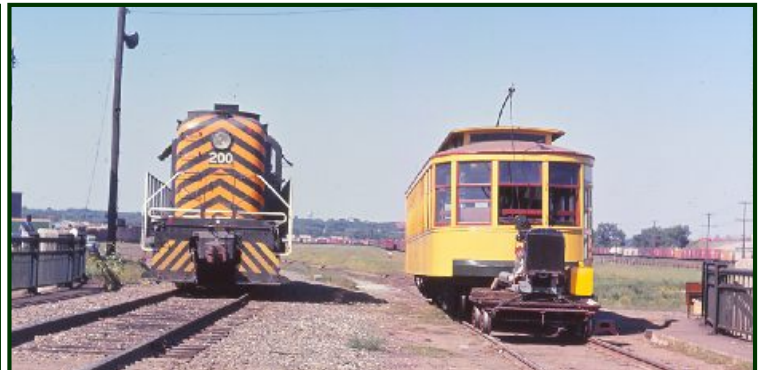
A Minn. Transfer Alco RS-3 locomotive was surprised to meet No. 1300 on the Transfer's University Avenue bridge. This was a test run in early May, 1963. Power supply was the "goat" gasoline-powered generator seen here.
