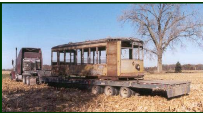
No. 28 arrived at Ken Albrecht's farm around 4:30 PM. For the next 2 hours, the crew used blocking to jack-up No. 28 so the trailer could pull out from under it. The crew then had to lower the car closer to the ground so it wouldn't tip over in a stiff wind.
