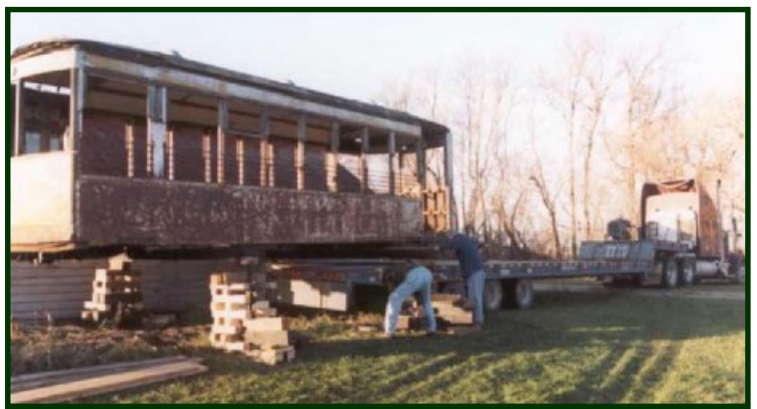
Bright & early Saturday morning (October 18, 2003) the truck arrives and loading and tie down begins. Note the body of No. 28 is way, way up in the air. The trailer bed was 40 inches off the ground so the bottom of the cross beams supporting No. 28 were about 45 inches off the ground.
