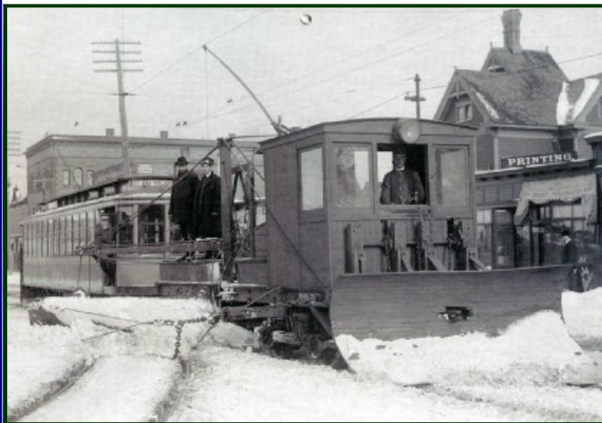
In 1905 a TCRT plow stops for a few minutes for the photographer on Nicollet Avenue just south of 31st Street in front of Nicollet Station. Everett C. Jones, a TCRT employee, is the Motorman shown in the cab. TCRT was required by its franchise to plow the streets on which it operated. A few years later the company built a fleet of more powerful and fully enclosed snow plows, capable of clearing a street in two passes. Note the open body where the wingman and Foreman must stand while operating—brrrrr. And, the front plow is made of wood slats!.
