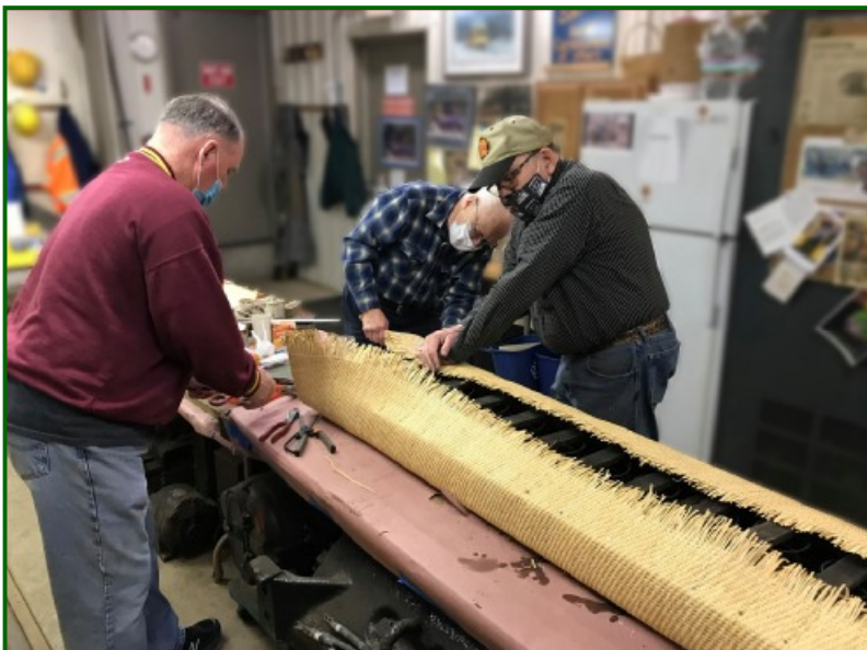
(ABOVE) Jack Bacon, Russ Isbrandt and John Prestholdt are putting new rattan on a bench seat for gate car No. 1239. They're doing this to return No. 1239 to its early 1920s look that we're striving for. This seat will remain natural and will be varnished rather than painted, which TCRT began to do in the 1920s. (LEFT) Here's the new Baker heater in its approximate location in the cab of No. 1239. You'll get the whole story on that perforated shield around the heater's smoke flue in an up-coming photo supplement. (Photos by Dennis Stephens)
