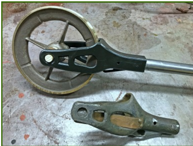
(LEFT) Twin City Rapid Transit had larger-than-normal trolley wheels which required larger trolley harps. The harp on the bottom is an original and the one on top is a plastic replica created by a 3D printer. We'll use the plastic harp as a pattern to cast a new harp in bronze or iron using the investment casting (lost wax) method. (Photo by Dennis Stephens)
