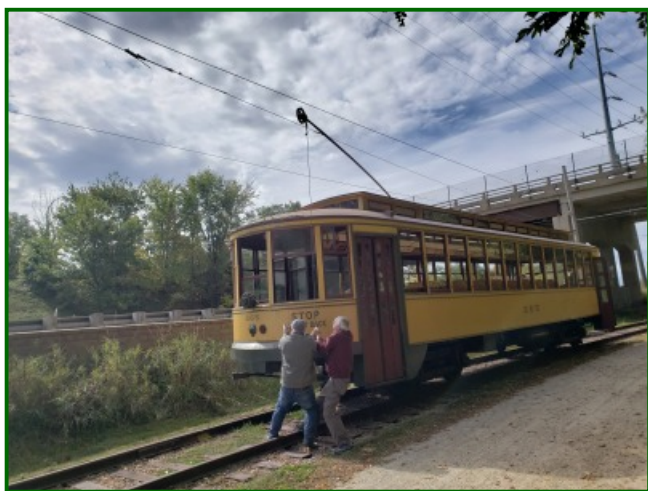
(ABOVE) We have some of the window "screens" that were mounted on the "pole side" of TCRT's standard cars so passengers couldn't stick arms or heads outside the car. Recently Karl Jones put one on No. 265 to show what they looked like and how they were mounted to the window posts. We don't put them on our cars primarily because they're ugly and we don't have enough of them for even one car. Note the winter storm window mounted on No. 265 to the right of the screen. (Photo by Karen Kertzman)
