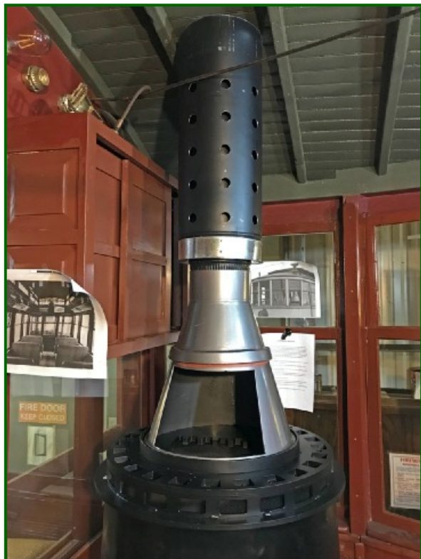
(ABOVE) Jack Bacon, Russ Isbrandt and John Prestholdt are putting new rattan on a bench seat for gate car No. 1239. They're doing this to return No. 1239 to its early 1920s look that we're striving for. This seat will remain natural and will be varnished rather than painted, which TCRT began to do in the 1920s. (LEFT) Here's the new Baker heater in its approximate location in the cab of No. 1239. You'll get the whole story on that perforated shield around the heater's smoke flue in an up-coming photo supplement. (Photos by Dennis Stephens)
