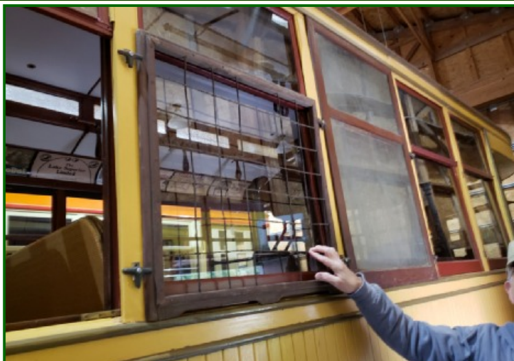
(ABOVE) We have some of the window "screens" that were mounted on the "pole side" of TCRT's standard cars so passengers couldn't stick arms or heads outside the car. Recently Karl Jones put one on No. 265 to show what they looked like and how they were mounted to the window posts. We don't put them on our cars primarily because they're ugly and we don't have enough of them for even one car. Note the winter storm window mounted on No. 265 to the right of the screen. (Photo by Karen Kertzman)
