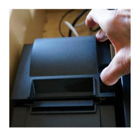
Remove the old roll of paper (or the empty spool) and drop in the new one as shown below, pulling the end up beyond the front of the lid. Close the lid.
