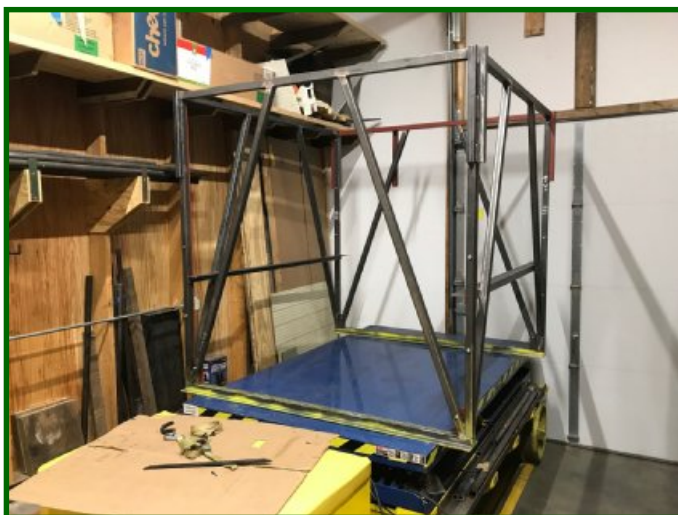
We're well on our way to having a good and accessible tower car at CHSL. (Above Left) Isaac Trockman is seen doing some finishing work on the new steel tower. (Aaron Isaacs photo) (Above Right) the tower is now on the scissors lift. Next step is to fabricate the platform and railings to the tower. (Dennis Stephens photo)
