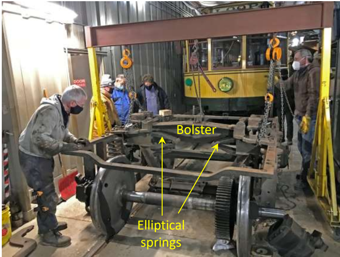
Lifting frame off wheels & axles; Karl Jones, Tom Schramm, Jim Willmore, Pat Cosgrove, Rob Mangels
