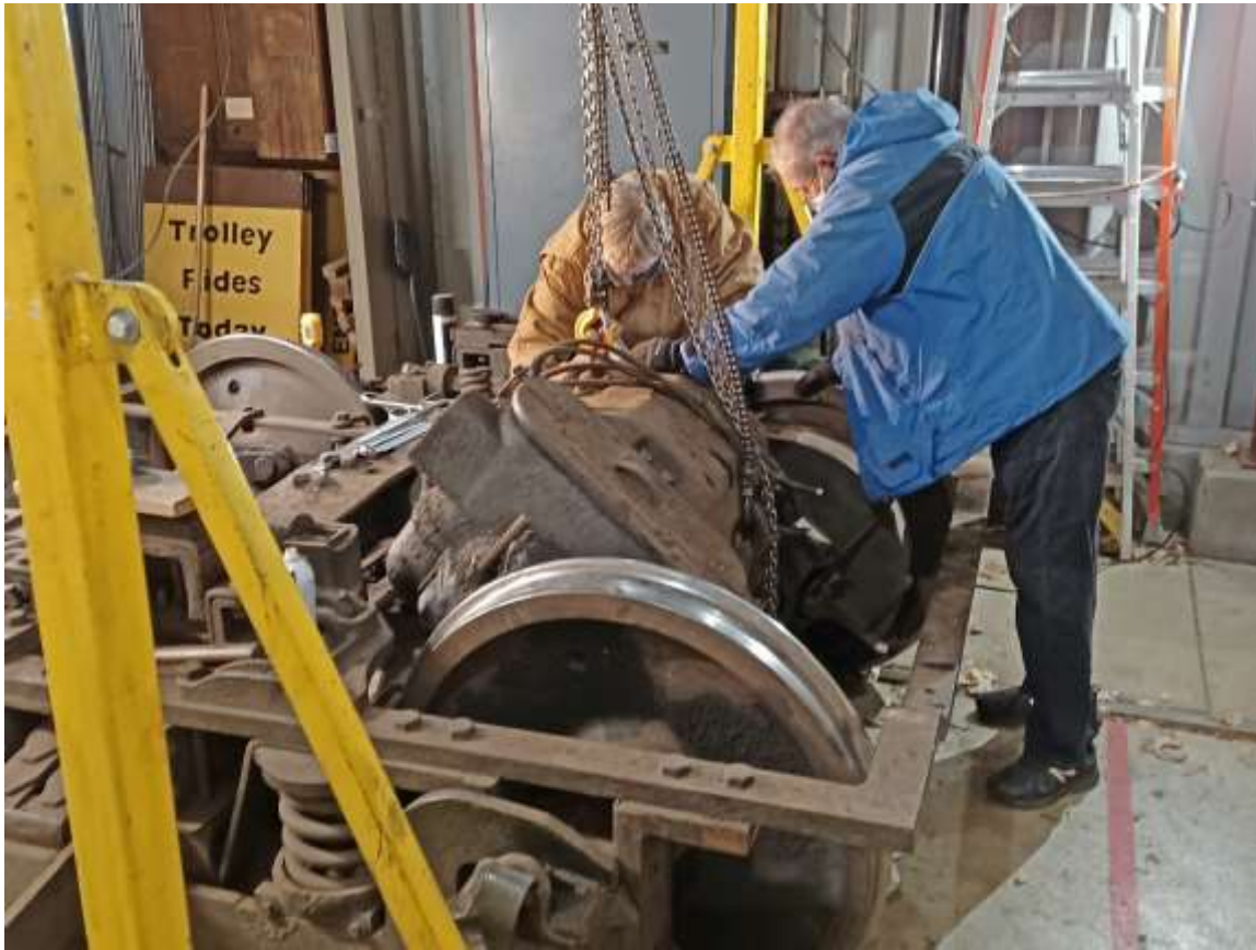
Tom Schramm and Jim Willmore pulling single motor from 1239 lead truck, former CTA L car trailer truck (K. Jones)
