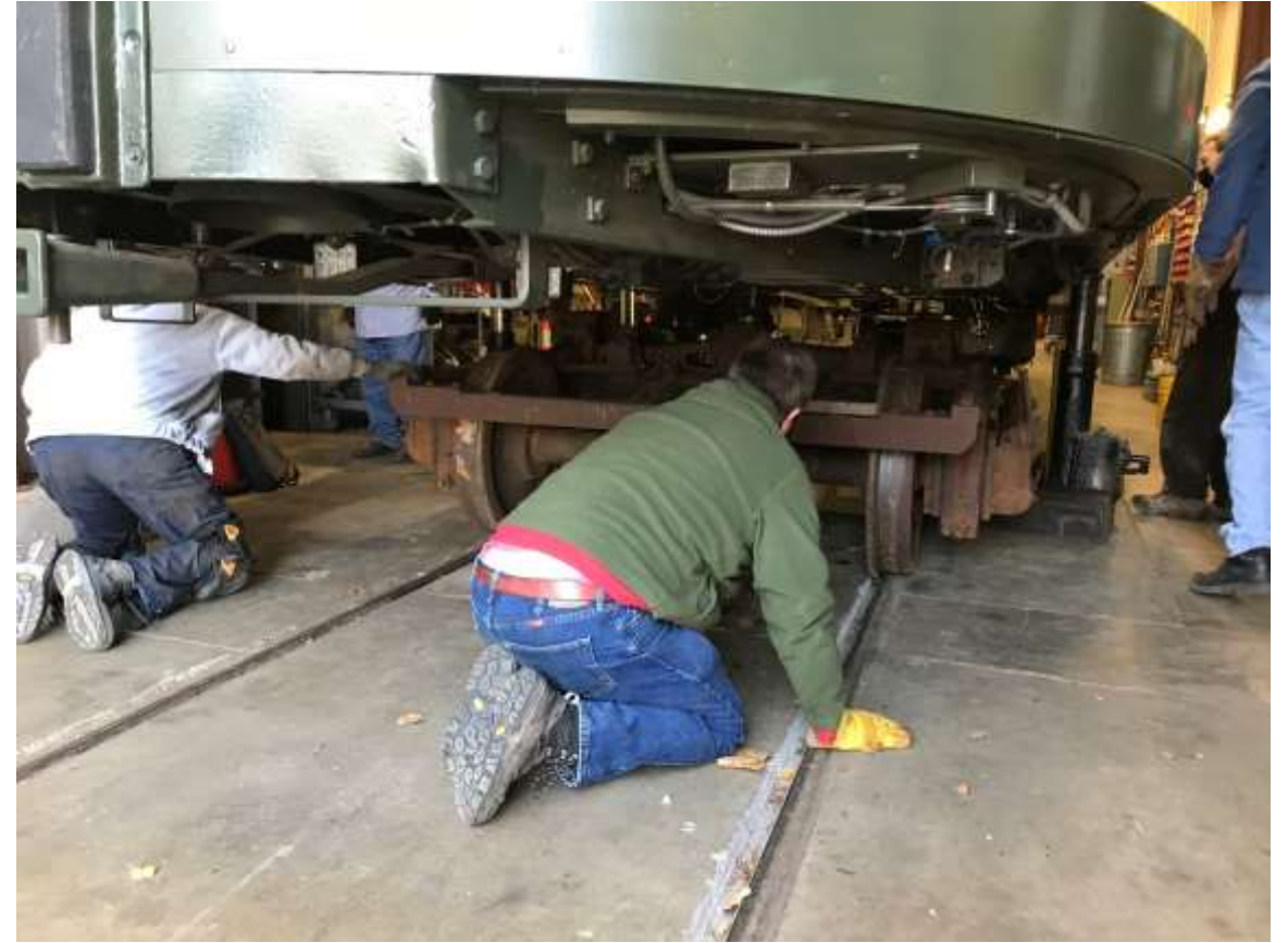
Karl and Ben position IRM shop truck under 1239. Center pivot has been reconfigured with parts from original 1239 truck
