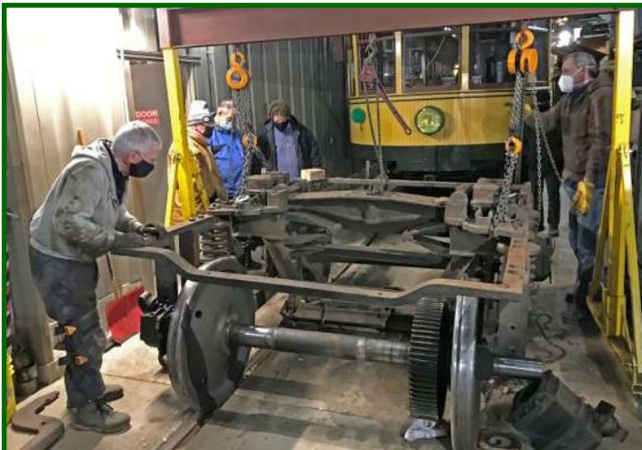
Disassembly begins. On this day, the CHSL shop crew taking the old CTA truck apart includes (L to R) Karl Jones, Tom Schramm, Jim Willmore, Pat Cosgrove & Rob Mangels . They have lifted the frame up so the axle and wheels can be rolled out.
