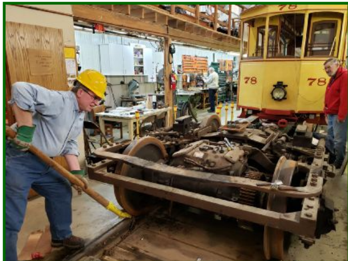
The ESL shop guys are working on one of the Baldwin trucks that are under Mesaba No. 10. Here we see Jerry Draeger (L) using a car mover to move the truck. Scott Heiderich is supervising and Steve Mages is working in the background. (Karen Kertzman photo)
