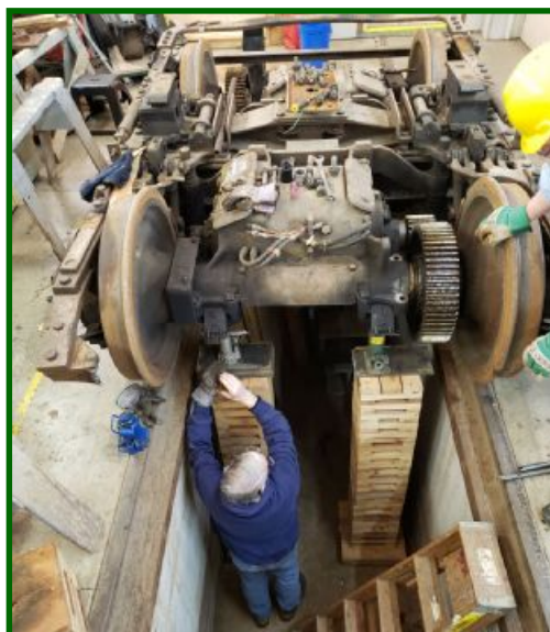
The ESL shop guys are working on one of the Baldwin trucks that are under Mesaba No. 10. Here we see Jerry Draeger (L) using a car mover to move the truck. Scott Heiderich is supervising and Steve Mages is working in the background. (Karen Kertzman photo)
