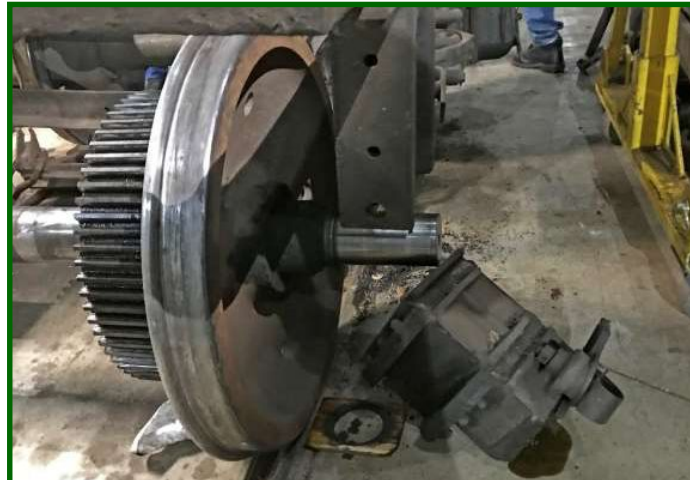
Here we see the axle and wheels being removed from under the truck frame. The end of the axle is called the journal and the boxy thing that's on the floor is the journal box.
