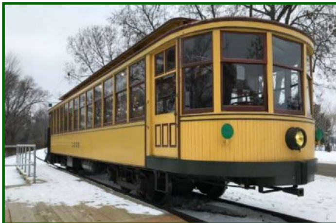
Shortly after No. 1239 was moved from ESL to CHSL, a test run was made to the north end of CHSL on December 8, 2018. The car could not run in regular service because the two motorized axles were not the correct track gauge. (All photos except as noted by Dennis Stephens)
