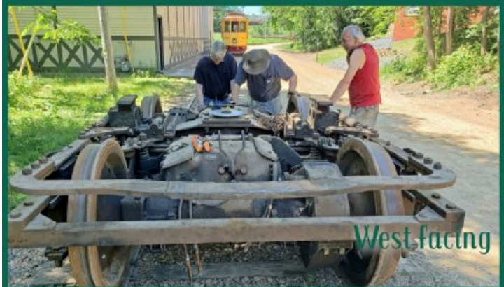
As part of correctly placing the trucks under Mesaba No. 10, one of them had to be turned around. In the above two pictures the curved brake bar is shown in front. Sometime between the two pictures, the magic of rotating the 12,000 pound truck happened! The crew was Howie Melco , Jim Kertzman and Scott Wardrope . (Photo by Karen Kertzman)
