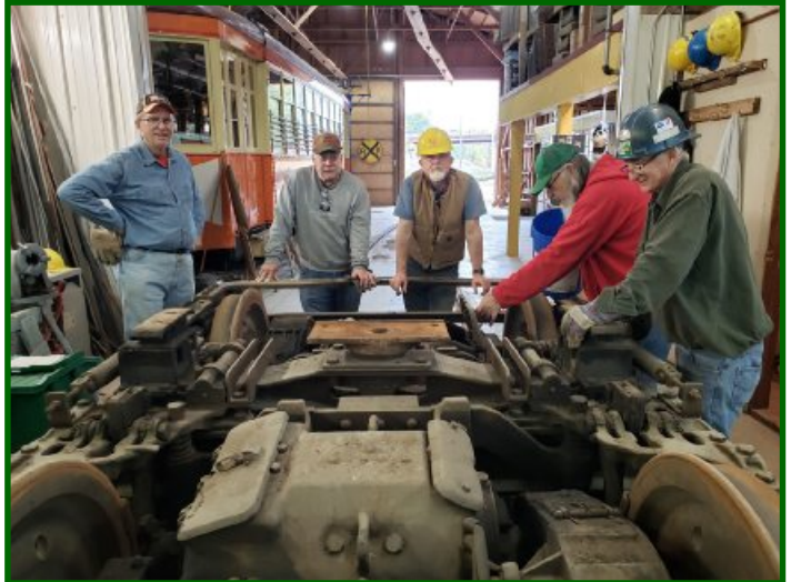
Here's (L to R) Jerry Draeger, Dick Zawacki, Howie Melco, Scott Heiderich and Scott Wardrope contemplating what's next for this Baldwin interurban power truck that will go under Mesaba Rwy No. 10. (Karen Kertzman Photo)
