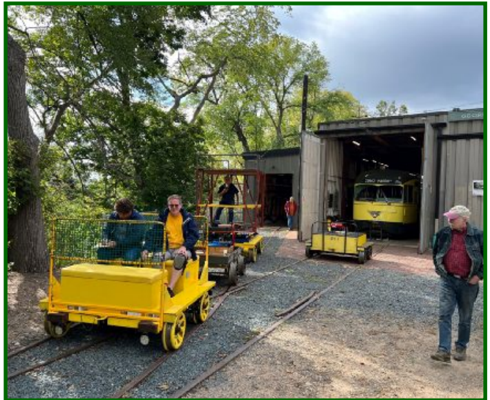
Here's a better photo of CHSL's new wire repair train going out for a test run. Pat Cosgrove (Left) and Jerry Betz are seated in the new battery-powered "turbo speeder" with Karl Jones standing on the new tower wagon. Bill Arends is on the right admiring the new equipment. In the background on the left is the entrance to the "speeder barn." Note that this door is much smaller than the regular carbarn doors. The new tower wagon was built with the working platform on a powered lift so the tower can be lowered from working height and fit through the smaller door. (Aaron Isaacs photo)
