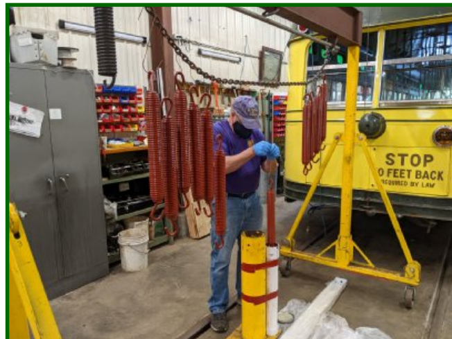
Dennis Stephens is seen here "painting" the brake release springs that will go on No. 1239's trucks. He's dipping the whole spring into a plastic pipe filled with the red oxide paint. Ingenious way to paint something long, eh? (Jim Vaitkunas photo)
