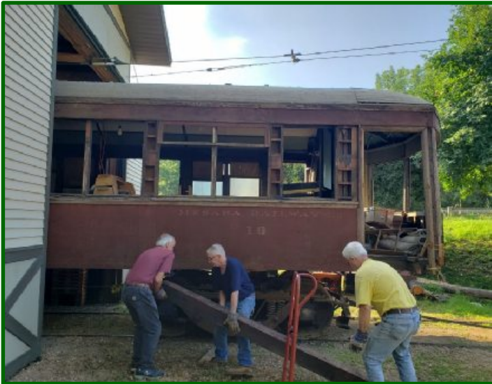
Jim Kertzman, Scott Wardrop, and Howie Melco prepare to put a tie under the car body to help stabilize and brace it during the move.
