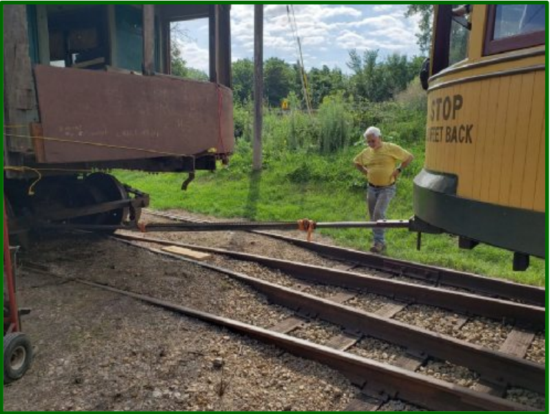
A tow bar was used to push Mesaba No. 10 into car barn track #2.
