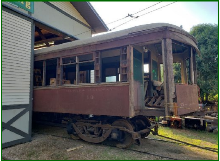
(Above) It was a tight squeeze to get Mesaba No. 10 out of the car barn, due to the misalignment of the track with the doors on track #3 and the curvature of the track outside the car barn. The car made it with less than an inch of clearance at one point. The misaligned track was one of the reasons for moving Mesaba No. 10.
