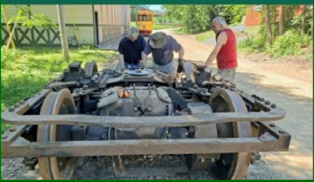
(Above) One truck needed to be rotated 180-degrees to get the brake rigging oriented so the two trucks will work correctly when the time comes to connect the car's brake rigging. With the help of a crane, Jim Kertzman (red shirt), Scott Wardrope (dark shirt), and Howie Melco (hat) supervised this operation. In the top picture one end of the truck faces east on the ESL tracks. In the bottom picture the same end of the truck now faces west (Right). Carl Floren helps Howie Melco align the carbody bolster to a hole in the front truck's bolster in preparation for installing the front kingpin. Other ESL shop crew volunteers are under the car moving the truck into the correct position to allow the kingpin to drop into place.
