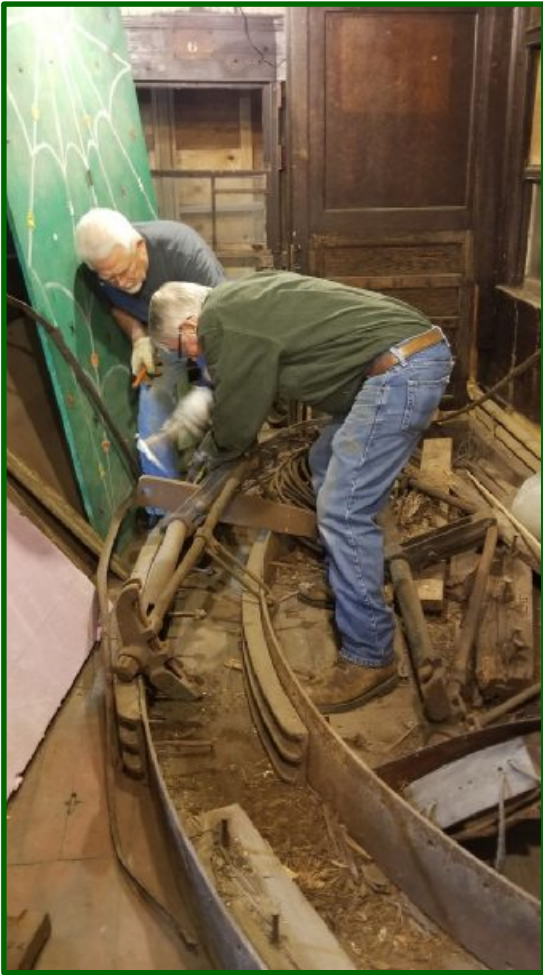
(Left) Scott Wardrope and Howie Melco are working on one of Mesaba No. 10's anti-climbers (a.k.a. "bumper") that was stored inside the car. Many other parts from the car and other cars, plus miscellaneous building materials, were haphazardly stored in the car. (Right) After scrap parts and unneeded building materials were removed from the car, and once the remaining materials were better organized, the original beauty and detail of the car's interior became apparent.
