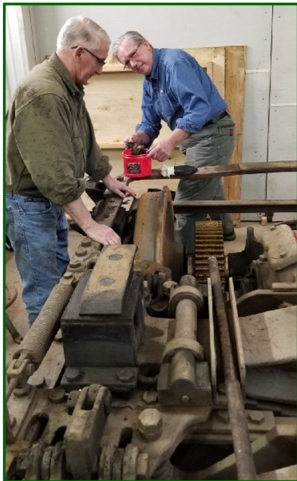
(Above) One of the two trucks stored under the Mesaba No. 10 carbody is pulled out from under it in preparation for cleaning and straightening in the warm barn. Notice the wooden "cribbing" that supports the car and holds it off the ground. Mississippi Valley Public Service Company No. 10, a single-truck streetcar, is in the background on track #2. It ran in Winona, Minnesota from 1914 to 1938 and awaits a rebuilt motor so it can enter service, hopefully in 2023.
