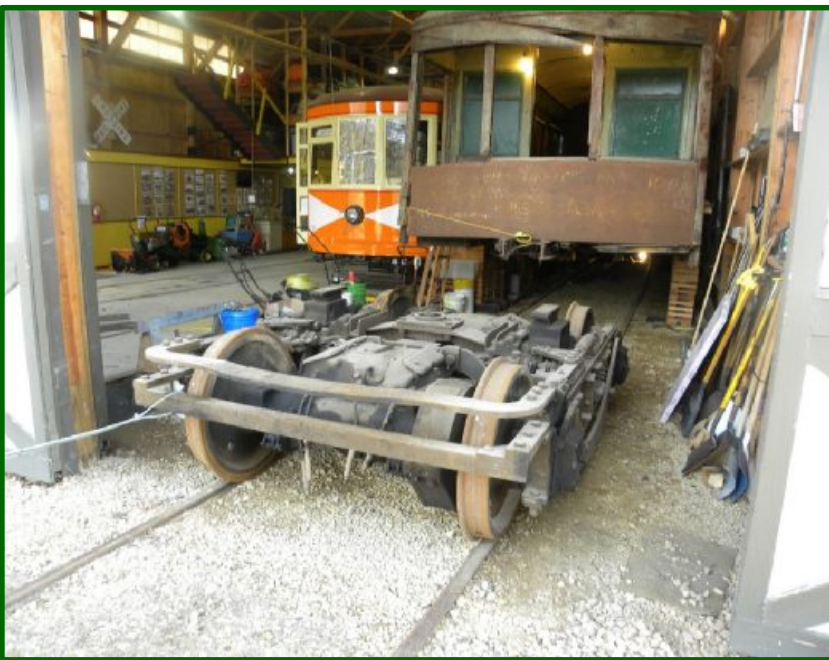
(Above) One of the two trucks stored under the Mesaba No. 10 carbody is pulled out from under it in preparation for cleaning and straightening in the warm barn. Notice the wooden "cribbing" that supports the car and holds it off the ground. Mississippi Valley Public Service Company No. 10, a single-truck streetcar, is in the background on track #2. It ran in Winona, Minnesota from 1914 to 1938 and awaits a rebuilt motor so it can enter service, hopefully in 2023.
