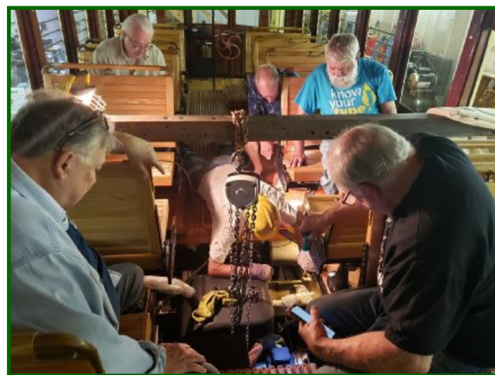
The ESL shop crew is lowering the MVPS (Winona lines) No. 10's motor into the correct position. (front to back) Chris Hawver, Dick Zawacki, Carl Floren (floor), Steve Mages, potential recruit, Michael Kimitch . (Karen Kertzman photo)
