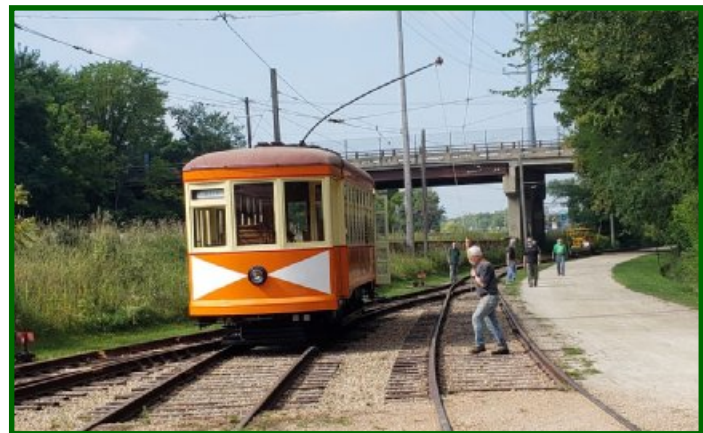
MVPS No. 10 returning to the carbarn following its first run with the repaired motor. That's Howie Melco turning the trolley pole around while the ESL shop crew is down the track by the mainline switch. (Karen Kertzman photo)
