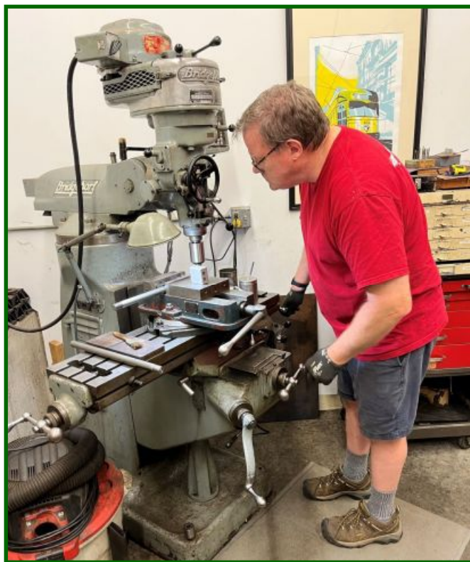
When you work to restore or repair old streetcars, you can't go to Home Depot to get parts—you have to make them in-house. In this photo we see Jerry Betz working on doing just that on a milling machine at CHSL. (Dennis Stephens photo)
