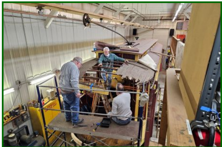
Repairs to the rear truck of TCRT No. 322 are on-going. In the left photo we see Jim Willmore and Mark Digre disconnecting the motor leads. In the right photo, the truck is out from under the car. That's Karl Jones standing on the left. Note that the motors are connected to the axle via a cardan shaft and gearbox which is much different from the "wheelbarrow" axle mounting of the electric motors on all the other streetcars our museum has in its collection. (Dennis Stephens photos)
