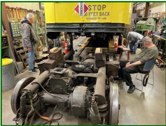
Repairs to the rear truck of TCRT No. 322 are on-going. In the left photo we see Jim Willmore and Mark Digre disconnecting the motor leads. In the right photo, the truck is out from under the car. That's Karl Jones standing on the left. Note that the motors are connected to the axle via a cardan shaft and gearbox which is much different from the "wheelbarrow" axle mounting of the electric motors on all the other streetcars our museum has in its collection. (Dennis Stephens photos)
