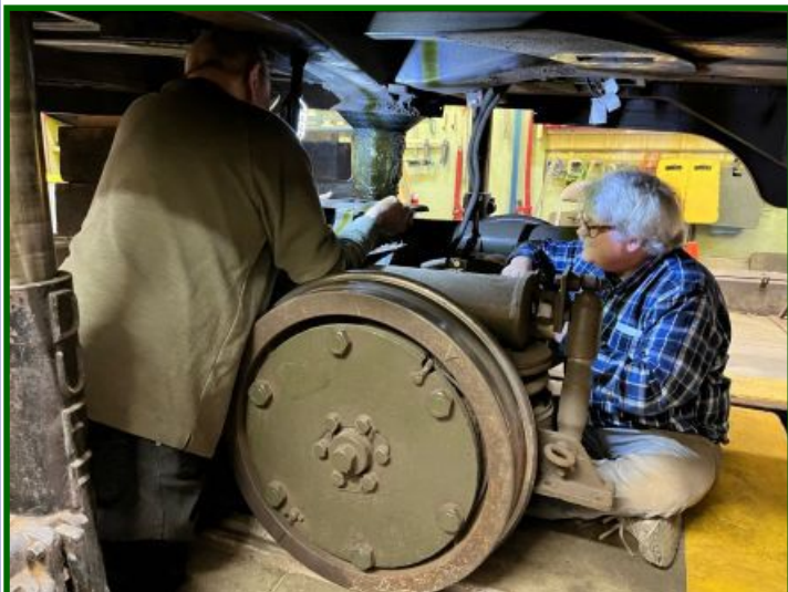
Repairs to the rear truck of TCRT No. 322 are on-going. In the left photo we see Jim Willmore and Mark Digre disconnecting the motor leads. In the right photo, the truck is out from under the car. That's Karl Jones standing on the left. Note that the motors are connected to the axle via a cardan shaft and gearbox which is much different from the "wheelbarrow" axle mounting of the electric motors on all the other streetcars our museum has in its collection. (Dennis Stephens photos)
