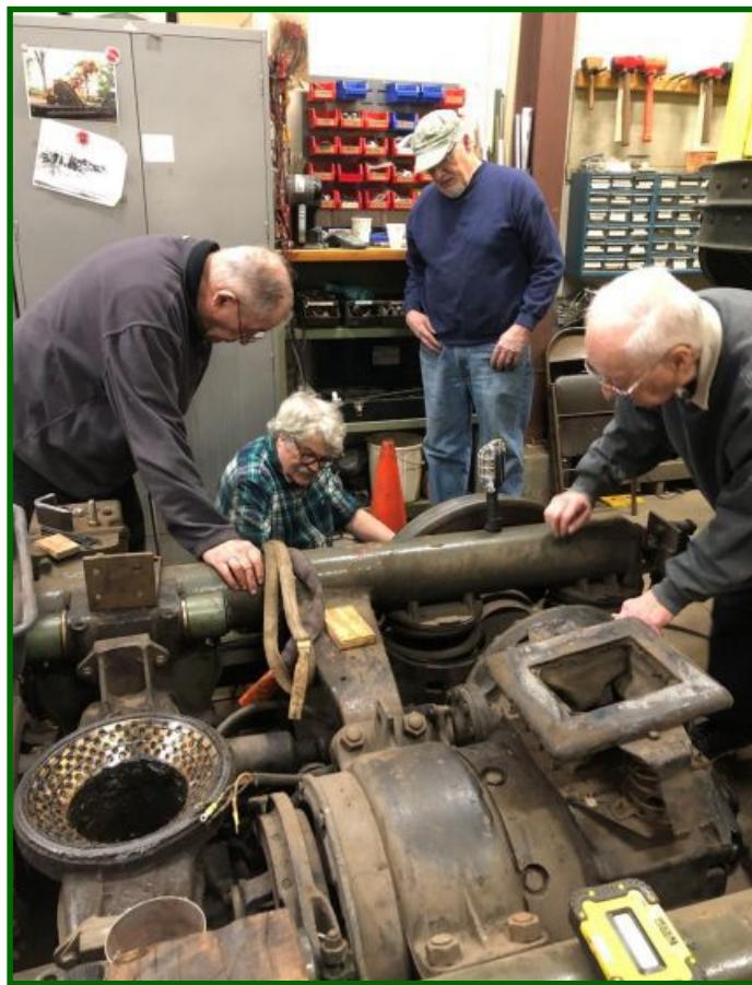
(L to R) Here's Jim Willmore, Mark Digre, Dennis Stephens and Russ Isbrandt working on the truck for PCC No. 322. (Bill Arends photo)
