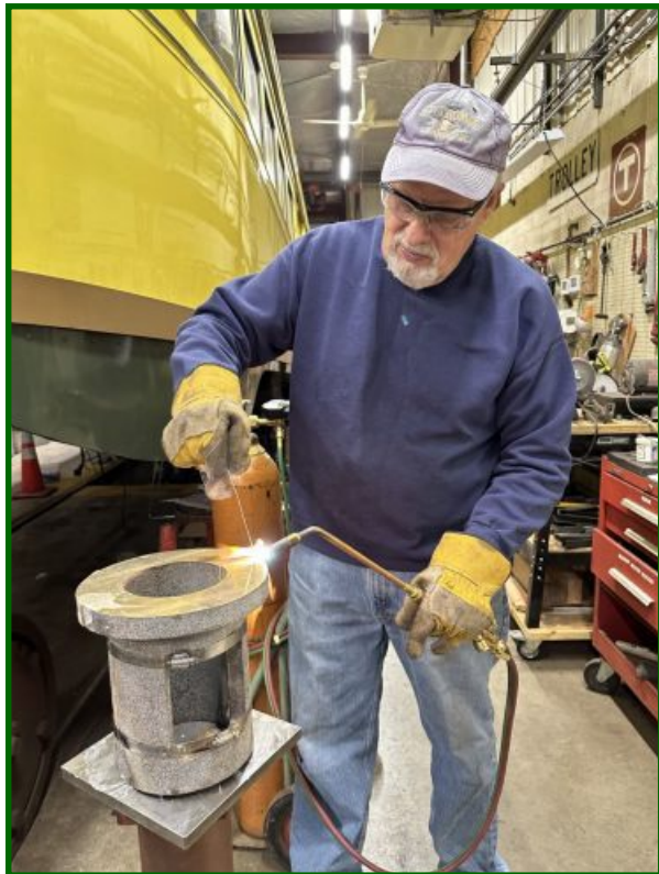
(Above) Dennis Stephens is seen here working on one of the motor support bearings for TCRT No. 1239.
