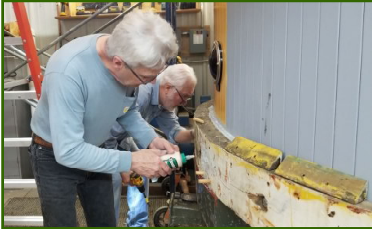
Mike Kimitch and Tom Heimer plugging the original screw holes with wood dowels in preparation for reattaching the metal bumper strip to No. 265. (Photo and caption by Karen Kertzman)
