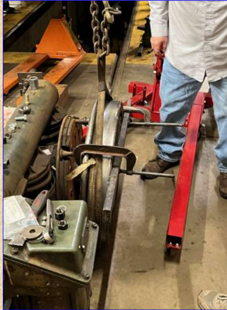
Bars and clamps maintain wheel assembly alignment; Tom Schramm and Mark Digre
