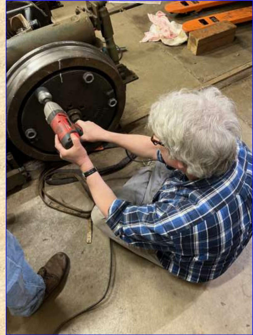
Bars and clamps maintain wheel assembly alignment; Tom Schramm and Mark Digre
