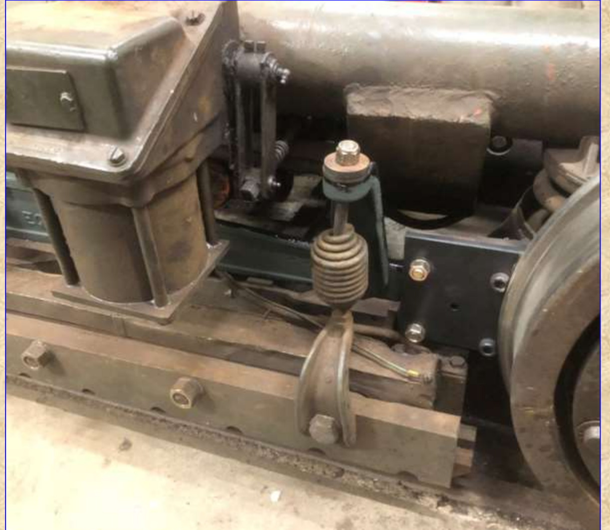
Aft end; L-bracket replaced by a simple plate
