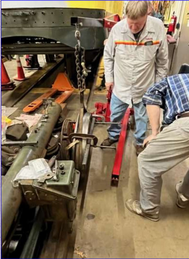
Bars and clamps maintain wheel assembly alignment; Tom Schramm and Mark Digre
